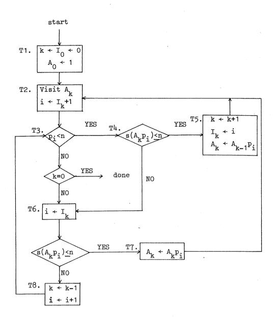
Figure 7.1. Flowchart of Algorithm T , which visits every node of the aliquot tree T[n] in the preorder sequence.
